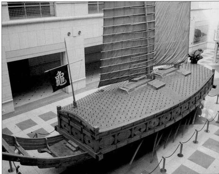
The turtle ship in the War Memorial Museum, Seoul, seen from above and showing the rows of spikes to discourage boarding. The flag bearing the character 'turtle' is also shown.
